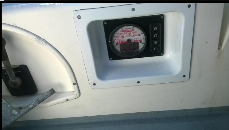
Above - Engine control panel on Sarico with fibreglass housing made using an oven dish as a mould!
