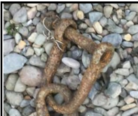
The shackle and monel seizing wire showing the loss of section between the pin and the body of the shackle after only 6 months of electrolysis in sea water.
